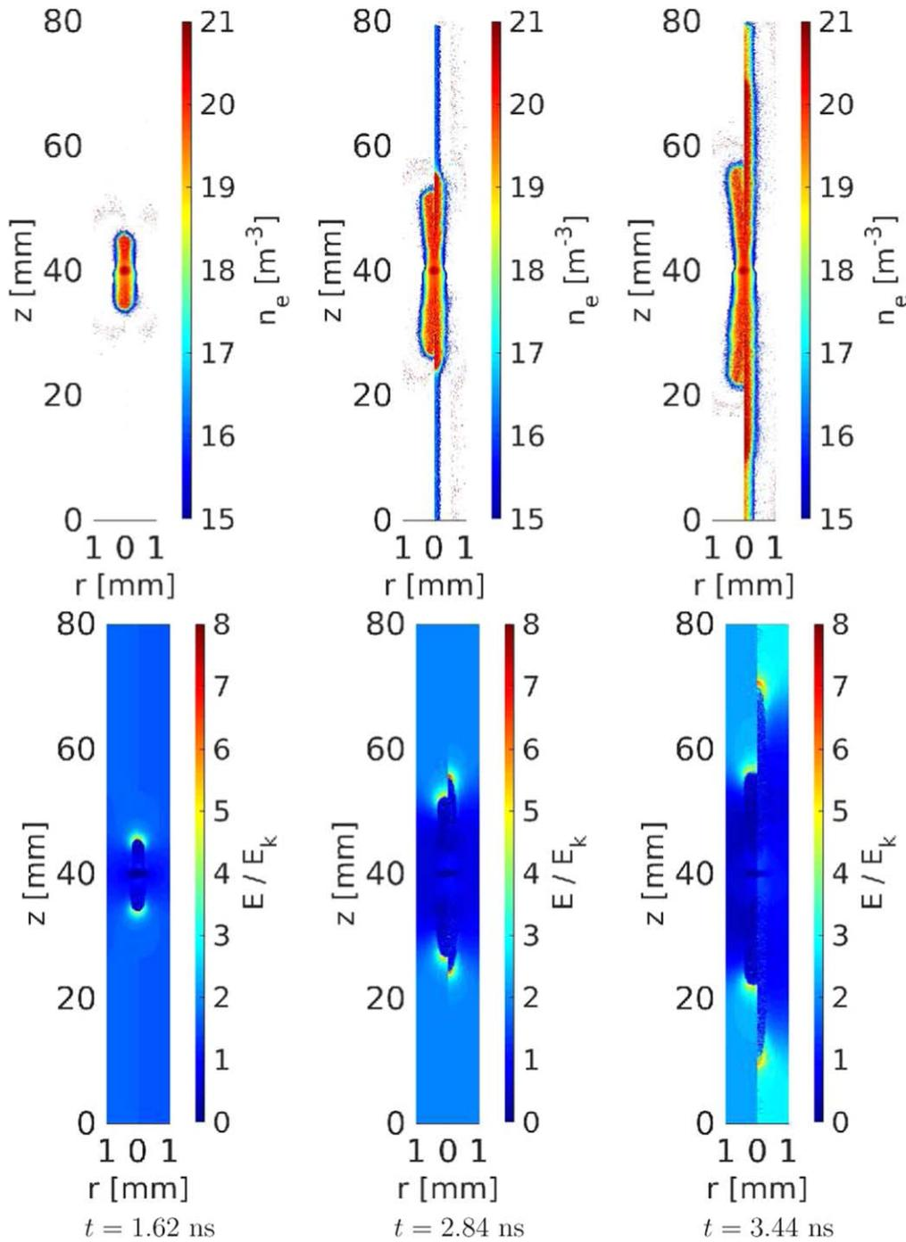
**Figure 6.** The electron density (top) and the electric field (bottom) in non-ionized air (left half of each panel) and in preionized air with  $n_{\text{pre},0} = 10^{12} \text{ m}^{-3}$  (right half) after different time steps.
