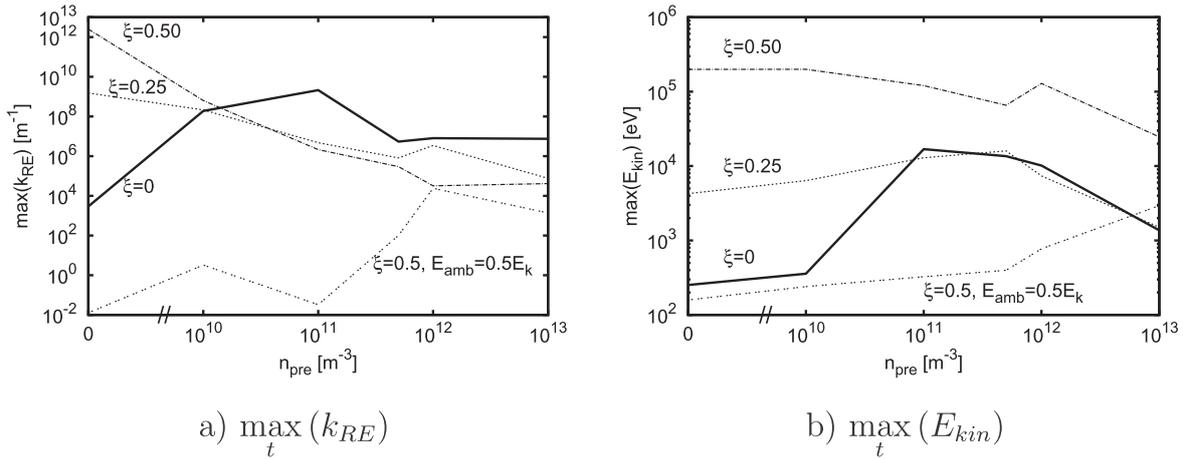
**Figure 8.** (a) The maximum number of runaway electrons per unit length,  $\max_t(k_{RE})$ , as a function of  $n_{pre,0}$  for  $\lambda_{pre} = \lambda_0$  and different levels  $\xi$  of air perturbation. (b) The maximum electron energy  $\max_t(E_{kin})$  for  $\lambda_{pre} = \lambda_0$  and different  $\xi$ . If not denoted otherwise, the ambient field here amounts to  $1.56E_k$ .
