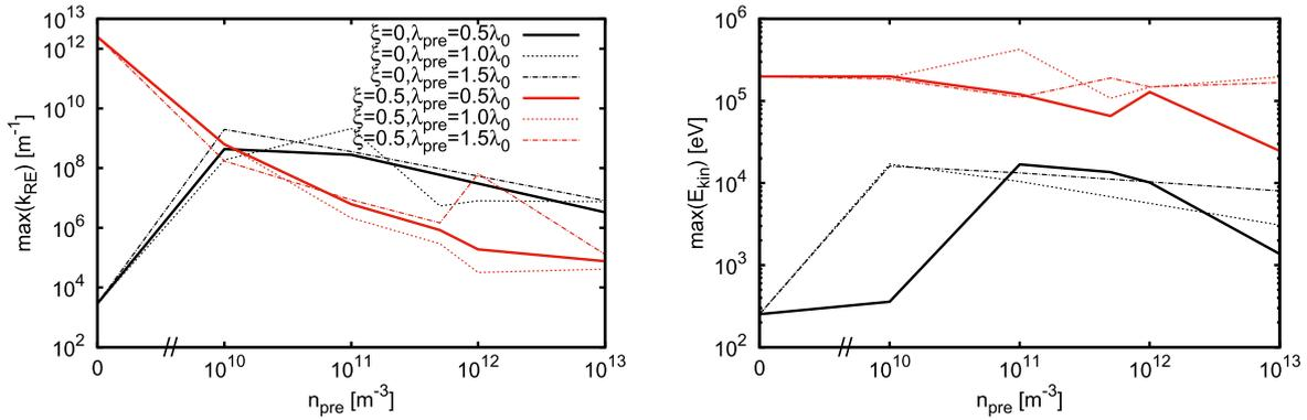
**Figure 11.** (a) The maximum number of runaway electrons per unit length  $\max_t(k_{RE})$  and (b) the maximum electron energy  $\max_t(E_{kin})$  for different channel radii  $\lambda_{pre}$  as a function of  $n_{pre,0}$ .
