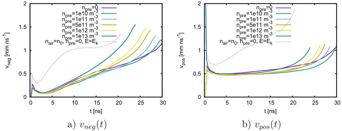
**Figure 9.** The streamer velocities of the negative (a) and positive (b) front as a function of time for  $\xi = 0.5$ ,  $E_{amb} = 0.5E_k$  and different levels  $n_{pre,0}$  of preionization. For comparison, the dotted line shows the streamer velocities in non-ionized and uniform air in an ambient field of  $E_k$ .
