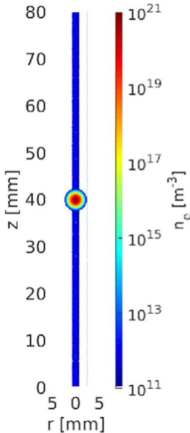
**Figure 2.** The simulation domain showing the electron density of the initial plasma patch (1) and of the preionization channel defined by equation (4)  $n_{\text{pre},0} = 10^{12} \text{ m}^{-3}$ . The preionized air channel is radially extended as widely as the initial electron-ion patch which is not visible because the colorbar is limited down at  $n_e = 10^{11} \text{ m}^{-3}$ .
